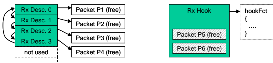
Fig. 4: buffers after omethHookCreate(..., &hookFct, 2)
