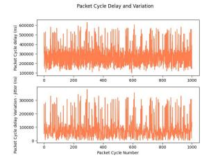
Figure 11c. Packet delay and jitter without TSN but with simultaneous best effort traffic
