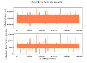
Figure 11d. Packet delay and jitter with TSN (802.1Qbv) and with simultaneous best effort traffic
