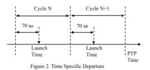
In this paper we use TSD to control time-aware scheduling. There are two reasons for this choice. First, it gives the user exact control over when the OPC UA packet shall be sent. Second, TSD, allows us to evaluate the effect of frame preemption (802.1Qbu/802.3br) on the maximum receive packet jitter.
