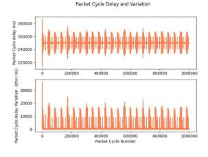
Figure 11a. Packet delay and jitter without TSN
