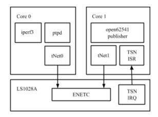
Figure 9. LS1028A core configuration
