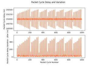
Figure 13. Packet delay and jitter with TSN (802.1Qbv+802.1Qbu) and with simultaneous best effort traffic
